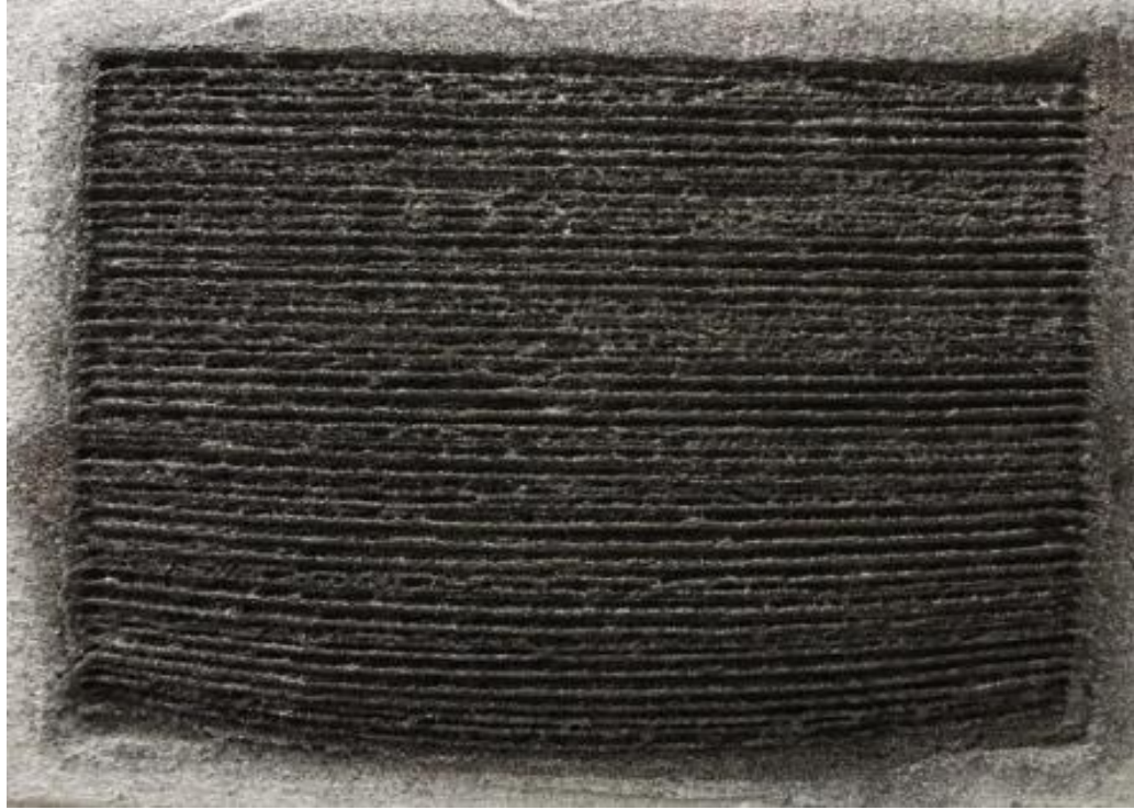
Figure 18. Shrinkage defect of SLS process
